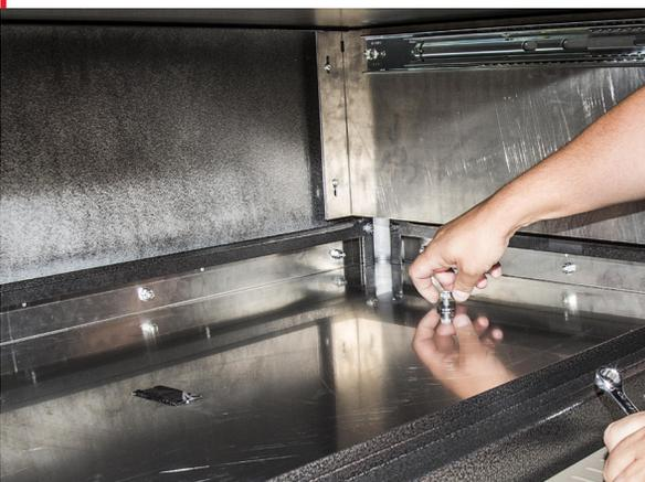
5. Reinstall drawer into CopBox Cabinet. make sure slides fit into roller bearing case securely without binding up.
