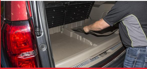
2. Remove factory cargo screws and pull out factory cargo floor.
